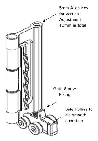
The double leaf roller incorporates a hinge which fixes the roller to the door sashes (top & bottom rollers) the rollers themselves have 10mm of adjustment (+&-5mm).
