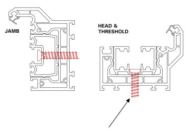
If this fixing is over tightened, it will distort the aluminium roller case and prevent the door from operating as it should.
