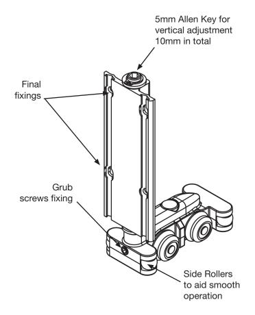
The single leaf roller is screwed directly in to the door sash euro-groove (top & bottom rollers) the rollers themselves have 10mm of adjustment (+ &- 5mm).
