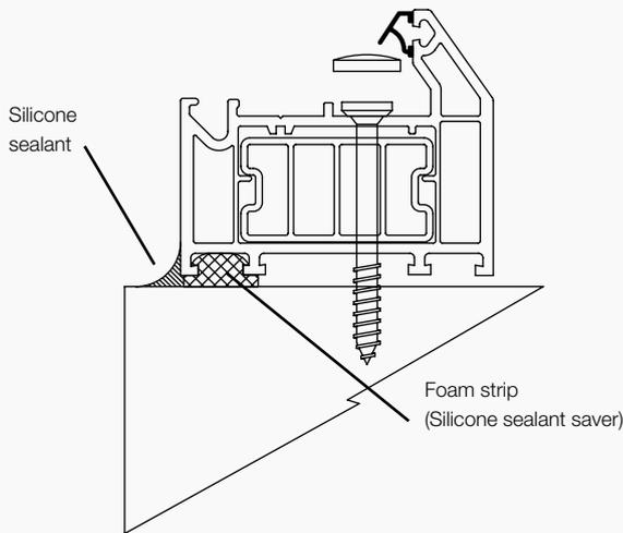
Having manufactured and installed the window so that there is a 5mm gap (approx.) between mainframe and masonry, it may be necessary to insert a flexible foam strip to form a base for the silicone sealant.
