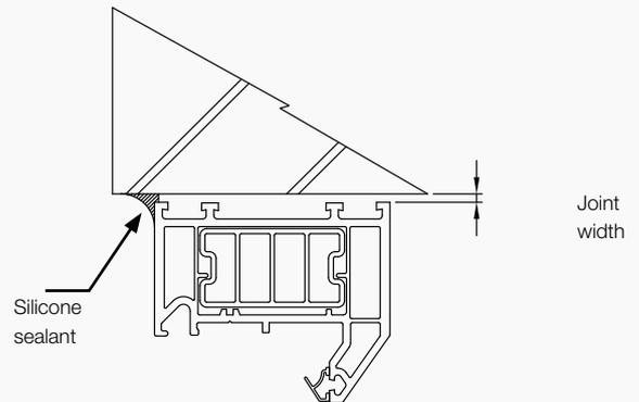
**B: joint width 6mm to 15mm.**
