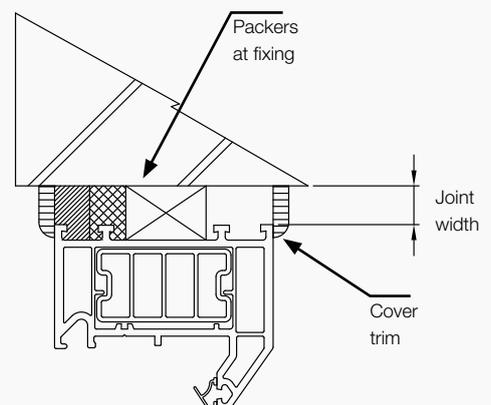
**EXAMPLES OF FRAME WEATHER SEALING**
